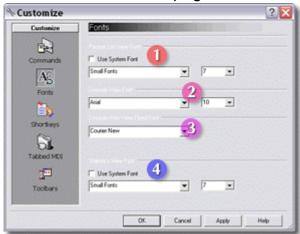
You can modify the fonts used by the Packet List View, the Decode View, the Hex View, and the Statistics View in this dialog.
