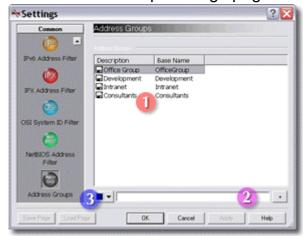
The Address Group Settings page is used to create and manage address groups. You can assign addresses to these groups on the different Address Filter Settings pages inside the Settings dialog. Address groups can be displayed in the Packet List by adding the MAC Grp. or Layer 3 Grp. columns on the Packet List Columns Settings page. And you can use Address Group statistics modules for the Statistics View, the Load over Time Statistics View, and for Reports.
