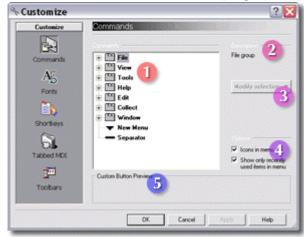
While this dialog is open, you can drag commands from its commands tree directly into toolbars and menus of the application. You can also move command entries and buttons in toolbars and menus to other locations. If you press the Ctrl key while dragging an item, it will be copied. If you move an item outside of a toolbar or menu, it will be deleted.
